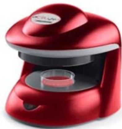
The new aCOLade colony counter is a reliable, easy-to-use device for the rapid manual counting of colonies on any agar in petri dishes. The versatile design accepts plates from 60mm to 150mm. A pressure sensor detects each count as the operator marks each colony with a pen and the LED readout displays the count. A 'back' button allows for incorrect counts to be rejected.
